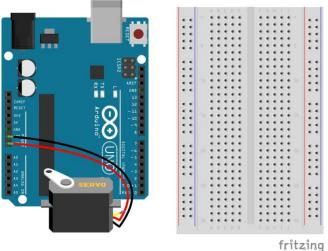
3. To finish hooking up the Servo, connect a white wire from 9 to the white (control) wire of the Servo (the wire in the diagram is yellow, but your wire may be white).
