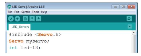
5. Now that you have named your Servo and LED, you're ready to write the Setup section of your Arduino program. Because you are using 2 components, a Servo and an LED, you need to setup both. You'll set up the Servo and the LED the same way that you did in the "Servo" and "LED Blink" activities, but this time you will put them both in the same program.
