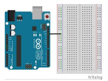
1. Start by connecting the black wire from | 2. Next, connect the red wire from pin 13 to any row on the breadboard (shown using row 16).
