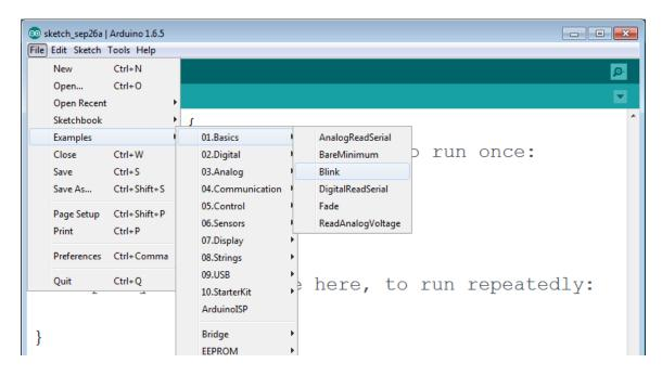
4. Finally, you need to "send" your text message. In Arduino, this is called "uploading," it is done by clicking the arrow button in the top left corner of your screen. Once this code uploads your LED should begin to blink.
