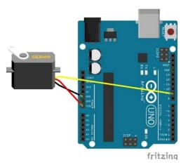
Connect the red wire to Vin, the black wire to GND, and the white wire to pin 9.
