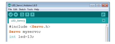
5. Now that you have named your Servo and LED, you're ready to write the Setup section of your program. Because you are using 2 components, a Servo and an LED, you need to setup both. You'll set up the Servo and the LED the same way that you did in the "Servo" and "LED Blink" activities, but this time you will put them both in the same program.
