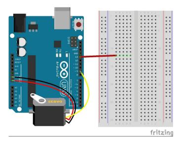
5. Next, connect a black wire from GND to the negative rail, or the blue lined column.
