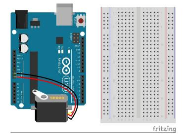
3. To finish hooking up the Servo, connect a white wire from 9 to the white (control) wire of the Servo (the wire in the diagram is yellow, but your wire may be white).
